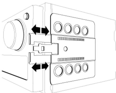
*The Kit includes mounting brackets (as shown on the picture), which need to be assembled on the aftermarket radio. KINDLY NOTE: these brackets allow to move the monitor in both directions. check the position out of the driver's seat.*
